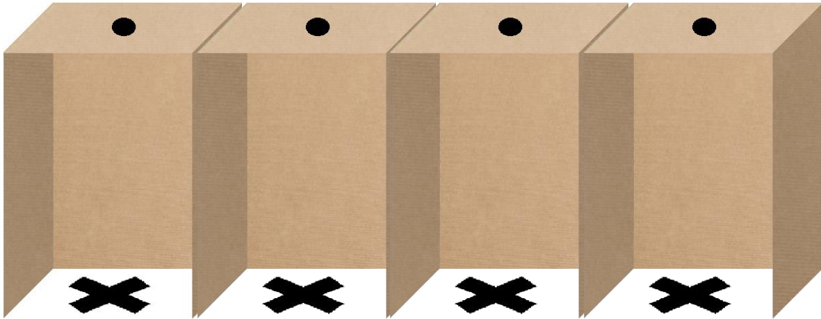
Figure 4 Cardboard arrangement – the framework for LED growth chambers. The black circles at the top indicate LEDs placement (cut with scissors) and the black crosses indicate the location of the samples.
