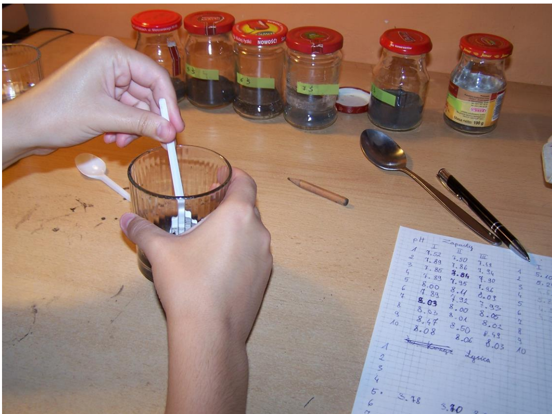
Pic. 10. Measuring the pH of soil.
